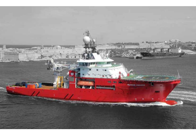
A purpose-built DNV Classed DP2 DSV with diesel-electric propulsion which was delivered in May 2010. The vessel features a fully built-in and classed 18-man single bell saturation diving system rated to 300m water depth, including a self-propelled hyperbaric lifeboat, and is designed for working in harsh environmental conditions.
